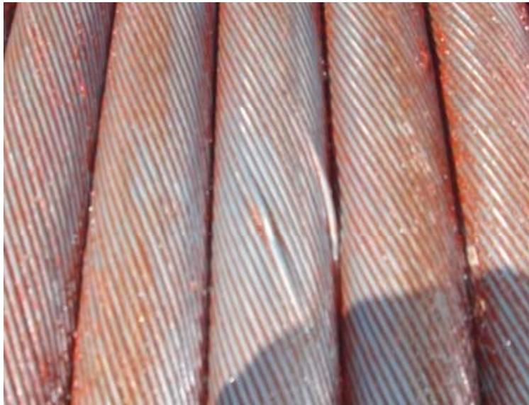
During BOS tests , the first failure of the sample was the breaking of a 24AWG conductor after 13429 cycles.
